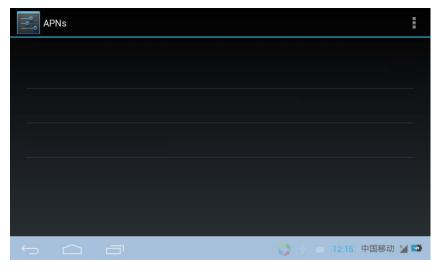
If there is some APNS, it means the device has detected SIM card.
