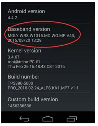
If it can check out the "Baseband version", it can detect the wireless module.
